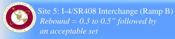
Pile: 18" Prestressed Concrete Piles Hammer: D36-32 single-acting diesel
